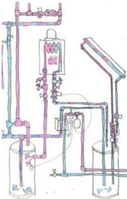
Set the output temp on the solar tank to about 170 degrees or so and when the pump cycles it won't cycle for long and the heated water will just flow straight through the DWH to the tempering tank and then out to the house through the tempering valve at 120 degrees.
