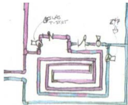
demanded by occupancy in the master bathroom. A bypass valve in the master bath vanity or similar discrete location allows the recirculation to bring hot water to the bath in the summer time with out heating the bath-room floor.
